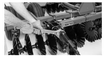
sure the roller basket assembly is level horizontatily with the disc (Photo 40).
